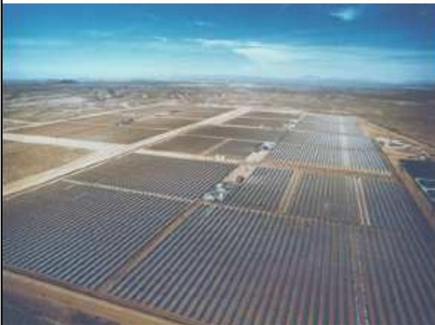
Figure 1: Aerial view of the five 30 MW<sub>e</sub> solar parabolic trough plants at Kramer Junction, California (Courtesy of KJC)
